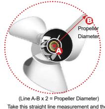
Take this straight line measurement and then double it to arrive at the Propeller diameter
